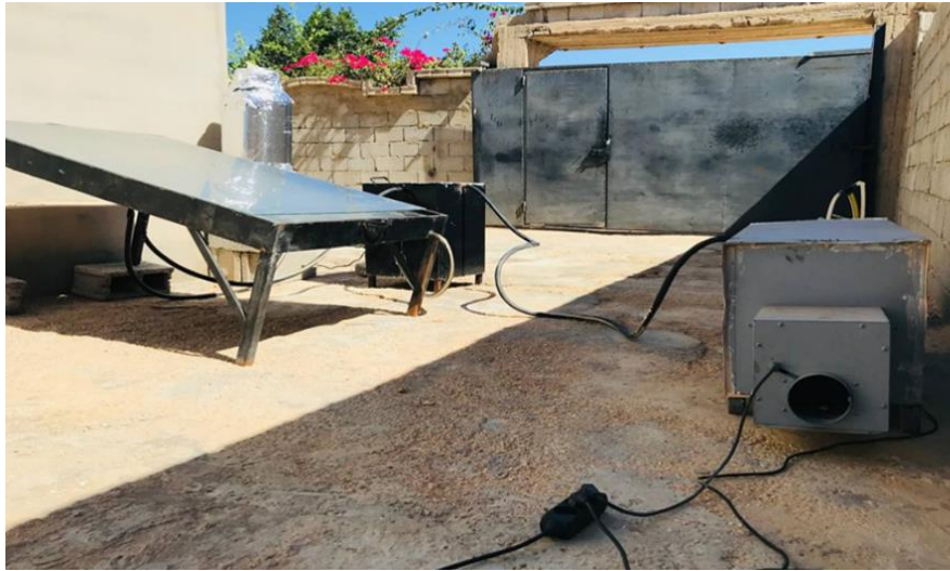
Figure 2. Photo of evaporative and condensate purification system.
